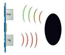
The equation of distance is distance =duration\* speed Here the speed is a speed of air  $340\mu m$  in one second. But this sensor used cm, so we need to convert speed to cm to become 0.0340cm.
