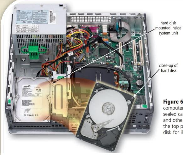
**Figure 6-3** The hard disk in a desktop computer is enclosed inside an airtight, sealed case inside the system unit. (In this and other hard disk photos in the book, the top plate is removed from the hard disk for illustration purposes.)
