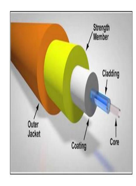
When the light enters one end of the optical fiber, it travels from a dense medium towards rare medium with a finite angle. The light ray hits the core-cladding interface with an angle greater than the critical angle and thus gets refelected at the interface due to total internal reflection. It suffers multiple total internal reflection the whole length of the fiber and finally emerges out of the other end of the fiber.
