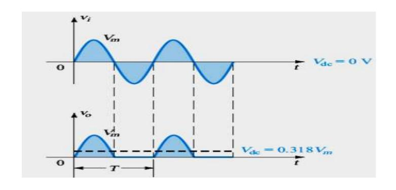
$$V_{AVG} = \frac{V_{p(out)}}{\pi}$$
