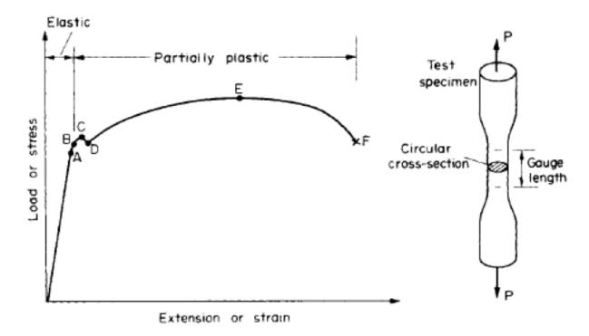
If a specimen of structural steel is gripped between the jaws of testing machine and the unit load or stress was plotted against unit elongation (or strain). The resulted diagram shown is called a stress-strain diagram
