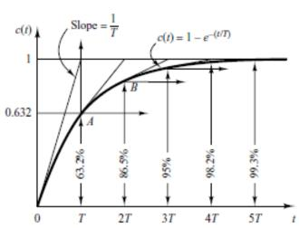
From Equation (4) we see that the slope of the response curve c(t) decreases monotonically from 1/T at t=0 to zero at  $t=\infty$ .
