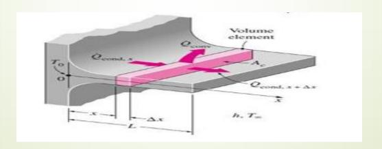
$$\begin{cases} Conduction \ Heat \\ Transfer \ Rate \ int \ o \\ The \ Element \ at \ x \end{cases} - \begin{cases} Conduction \ Heat \\ Transfer \ Rate \ from \\ The \ Element \ at \ x + \Delta x \end{cases} = \begin{cases} Convection \ Heat \\ Transfer \ Rate \ from \\ The \ Element \end{cases}$$
