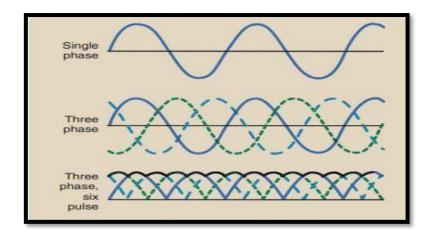
• High-frequency generators produce a nearly constant potential voltage waveform, improving image quality at lower patient radiation dose.
