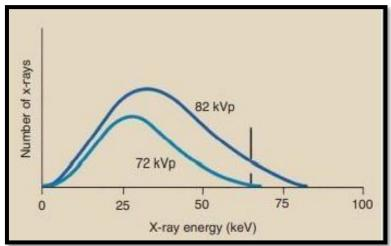
A change in kVp has no effect on the position of the discrete x-ray emission spectrum
