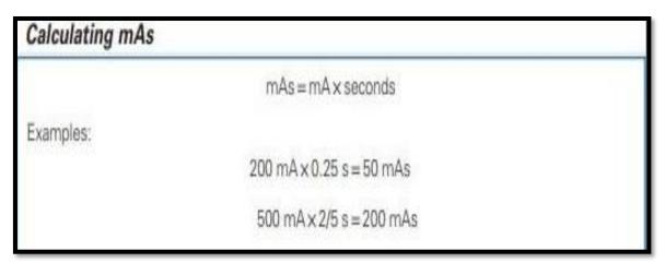
A change in mA or mAs results in a proportional change in the amplitude of the x-ray emission spectrum at all energies.
