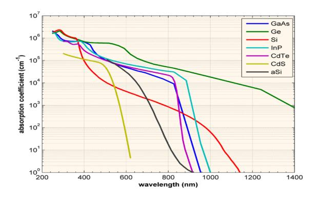
The absorption coefficient,  $\alpha$ , in a variety of semiconductor materials at 300K as a function of the vacuum wavelength of light.
