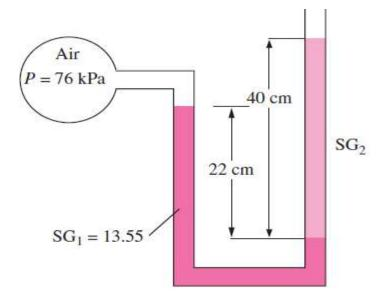
Q37/Consider the system shown in Fig. If a change of 0.7 kPa in the pressure of air causes the brine–mercury interface in the right column to drop by 5 mm in the brine level in the right column while the pressure in the brine pipe remains constant, determine the ratio of *A*2/*A*1
