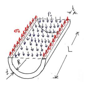
Force due to internal pressure =  $p^*$  Area
