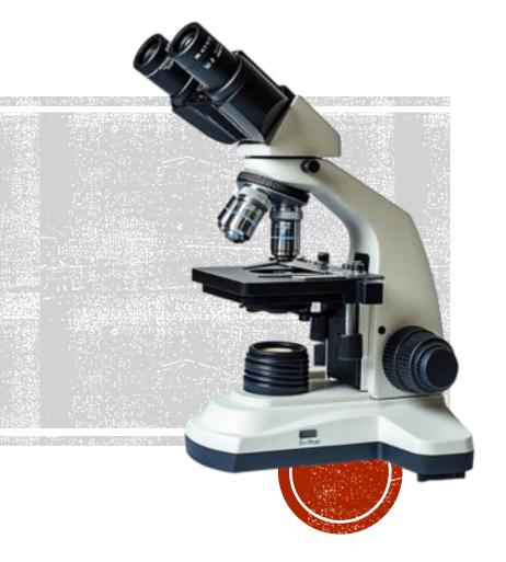
Microscopes are instruments that are used in science laboratories, to visualize very minute objects such as cells, microorganisms, giving a contrasting image, that is magnified. Microscopes are made up of lenses for magnification, each with its own magnification powers. Depending on the type of lens, it will magnify the specimen according to its focal strength.
