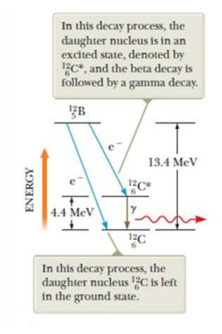
**Figure 5** An energy-level diagram showing the initial nuclear state of a <sup>12</sup>B nucleus and two possible lower-energy states of the <sup>12</sup>C nucleus.
