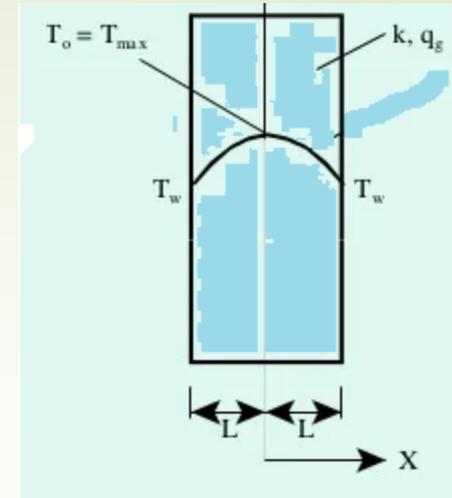
$$\rightarrow T_w = -\frac{\ddot{g}L^2}{2k} + C_2 \rightarrow C_2 = \frac{\ddot{g}L^2}{2k} + T_w$$
