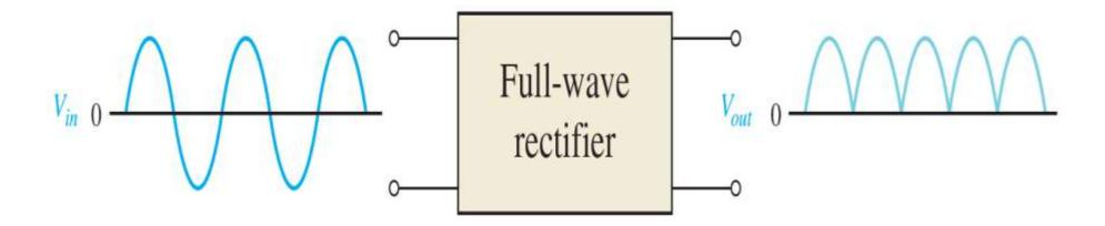
The average value for a full-wave rectified output voltage is twice that of the half-wave rectified output voltage, expressed as follows:
