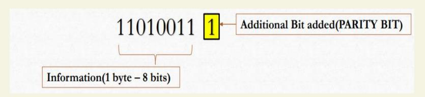
2. There are **two ways** to generate a Single parity bit: One is called **Even parity** and the other is **Odd parity**.
