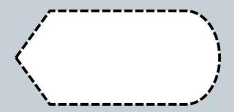
• Indicates a process flow step where information is displayed to a person (e.g., PC user, machine operator).
