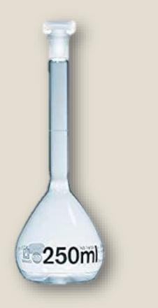
A volumetric flask is a key lab tool made of glass, calibrated to hold a precise volume of liquid at a specific temperature. It comes in various sizes and is mainly used in chemistry labs for preparing standard solutions.
