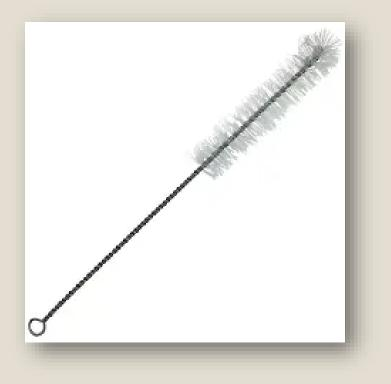
used for cleaning test tubes and narrow mouth laboratory glassware, such as graduated cylinders
