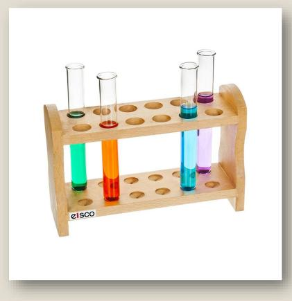
used to hold upright multiple test tubes at the same time.
