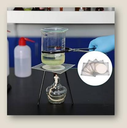
Wire gauze is a sheet of thin metal that has net-like patterns or a wire mesh with a ceramic center. The gauze is placed on the tripod stand between the Bunsen burner and the glassware to support the beakers, flasks, or other glassware during heating
