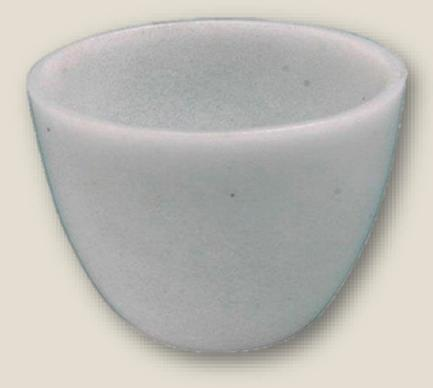
crucible is a cup-shaped piece of laboratory equipment used to contain chemical compounds when heating them to very high temperatures. The receptacle is usually made of porcelain or an inert metal.
