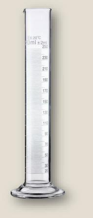
is a common piece of laboratory equipment used to measure the volume of a liquid.
