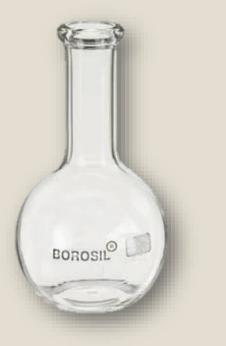
is used as a container to hold liquids. A Florence flask has a round body, a long neck, and often a flat bottom. It is designed for uniform heating, boiling, distillation and ease of swirling; it is produced in a number of different glass thicknesses to stand different types of use.
