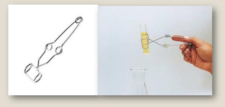
It is used for holding a test tube in place when the tube is hot or should not be touched
