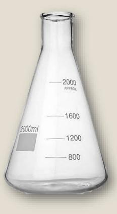
tool usually made of glass consists of a flat bottom, a tapered neck, a conical body, and an opening that can be closed by a stopper. It was named after its inventor, Emil Erlenmeyer. It is used to collect, store, and approximate measurement of liquid samples
