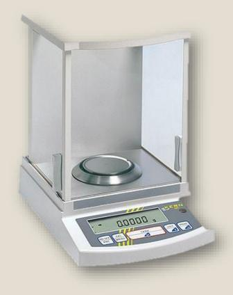
Analytical balances are an extremely accurate laboratory balance created to precisely measure the mass of an object.
