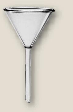
used in chemistry and other scientific experiments for funneling liquids or powders into containers with slim openings.
