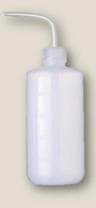
used to rinse various pieces of laboratory glassware, such as test tubes and round bottom flasks
