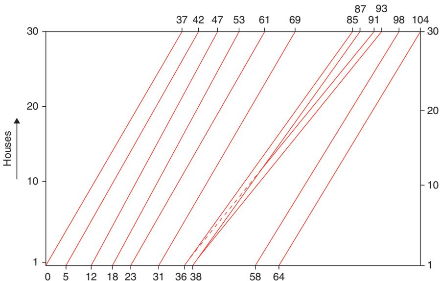
**Figure 2** The Line-of-Balance Schedule for the construction of the houses.
