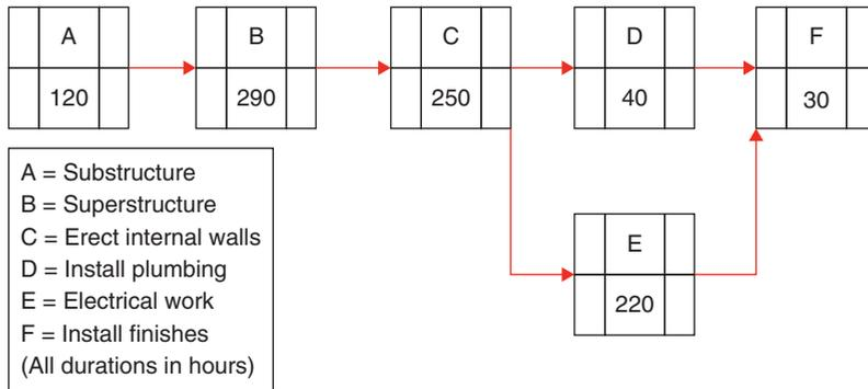
**Figure 1** The construction plan for each house.
