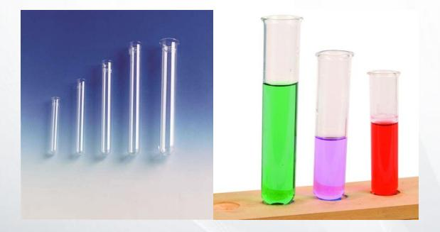
**Test Tube** Used to hold and mix liquids.
