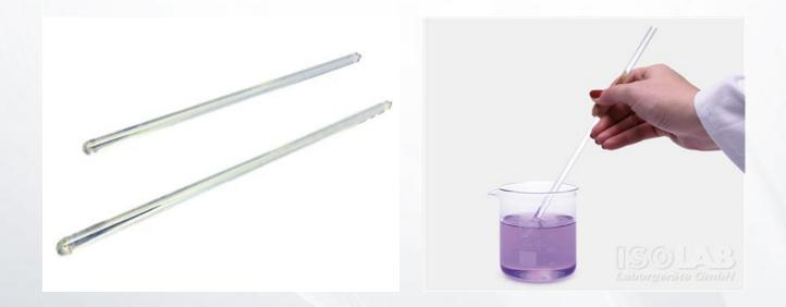
**Stirring Rod** Used for stirring and mixing
