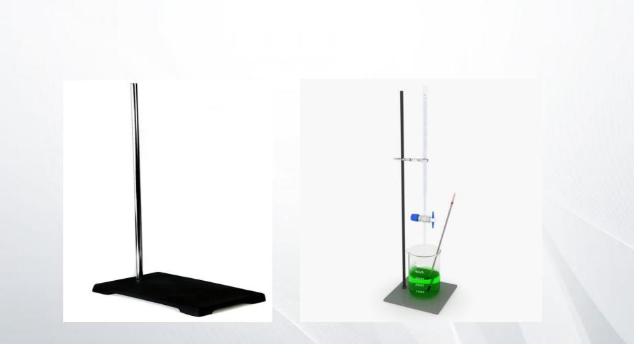
**Ring Stand** Used to hold or clamp laboratory glassware and other equipment in place, so it does not fall down or come apart.
