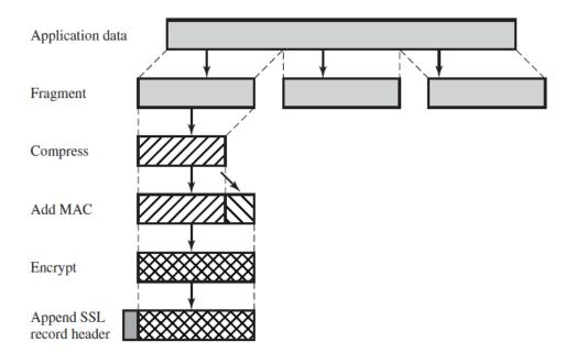
Figure /SSL Record Protocol Operation
