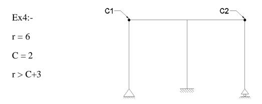
The frame is unstable because of internal geometric instability
