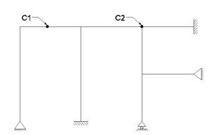
r > C+3, the frame is stable& indeterminate 5<sup>th</sup> degree.
