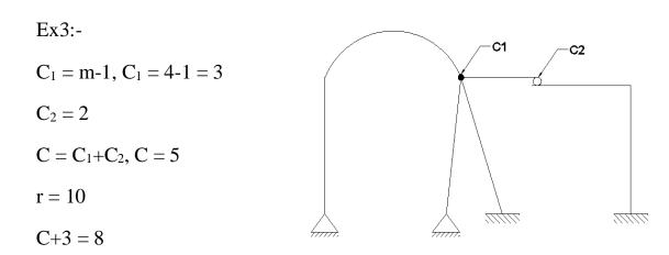
r > C + 3, the frame is stable & indeterminate  $2^{nd}$  degree.
