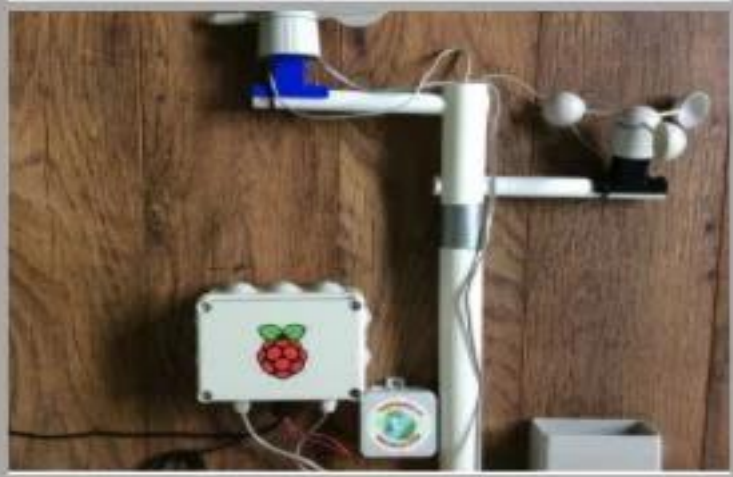
RASPBERRY PI WEATHER STATION
