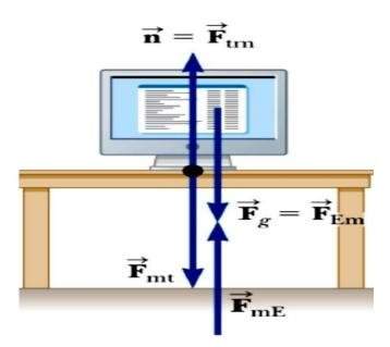
• Normal means perpendicular, in this case The action (Earth on monitor) force is equal in magnitude and opposite in direction to the reaction force, the force the monitor exerts on the Earth.
