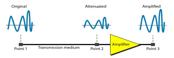
To show that a signal has lost or gained strength, engineers use the unit of the *decibel*. The **decibel** (**dB**)*measures the relative strengths of two signals or one signal at two different points*. Note that the decibel is negative if a signal is attenuated and positive if a signal is amplified.
