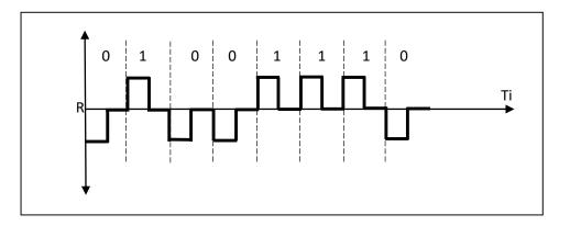
The main *disadvantage* of RZ encoding is that it requires two signal changes to encode one bit and therefore requires more bandwidth.
