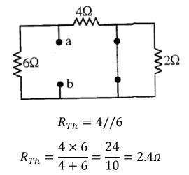
Step 2: find  $V_{Th}$  which is the voltage across the 6  $\Omega$  resistance
