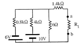
Sol: Step 1. Find R<sub>Th</sub> by replace the voltage source with short circuit
