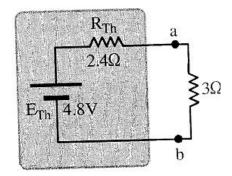
Example 5: Find the Thevenin equivalent to the circuit at terminals a and b
