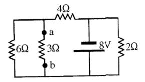
Sol: Step 1. Find  $R_{\text{Th}}$  by replace the voltage source with short circuit
