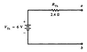
Example 2: To the circuit of Example 1, add a resistor load  $R_L$  of 3.60 and find the current  $I_L$  through the load and voltage  $V_L$  across the load.
