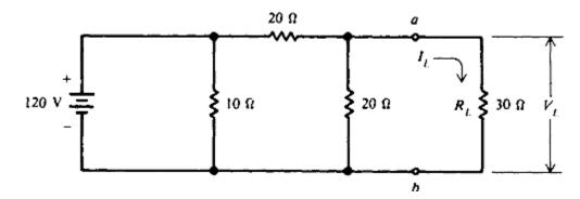
**Sol:** Step 1.Find R <sub>Th</sub>. Remove the load R<sub>L</sub>. Short-circuit the voltage source of 120V. Short-circuiting the battery also short-circuits the  $10\Omega$  resistor, leaving two  $20\Omega$  resistors in parallel.
