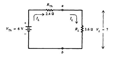
$$I_L = \frac{V_{Th}}{R_{TH} + R_L} = \frac{6}{2.4 + 3.6} = \frac{6}{6} = 1 \text{ A}$$
