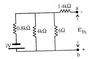
The resistance (1.4k  $\Omega$ ) neglected because the circuit is open. So  $V_{Th}$  is the voltage across the 6  $\Omega$  resistance
