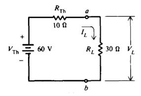
$$I_L = \frac{V_{Th}}{R_L + R_{Th}} = \frac{60}{30 + 10} = \frac{60}{40} = 1.5 \text{ A}$$
