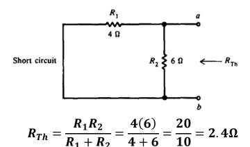
Find  $V_{Th}$ .  $V_{Th}$  is the voltage across terminals a and b, which is the same as the voltage drop across resistance  $R_2$ .
