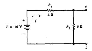
Sol: Step 1. Find RW. Short-circuit the voltage source V = 10V.  $R_1$  and  $R_2$  are in parallel.
