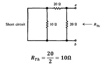
Step 2: Find  $V_{Th}$ . The two  $20\Omega$  resistors are in series across the 120-V line. Since the
