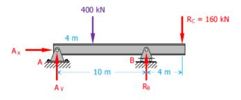
Example No. 3: Determine the horizontal and vertical components of reaction on the member at the pin A, and the normal reaction at B in Figure.
