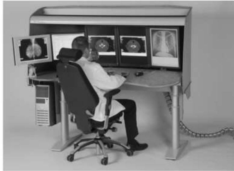
Fig. 4.3 A reading room as part of a PACS displays images on monitors instead of light boxes. Active and passive components of the depicted system control the lighting situation
