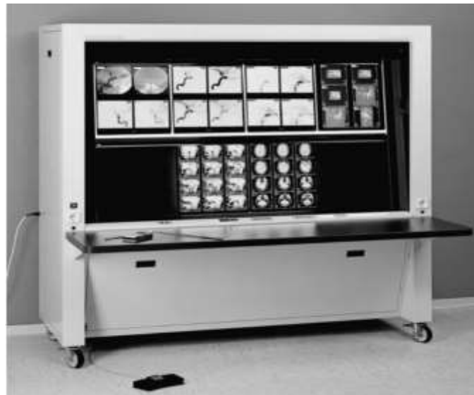
Fig 4.2 Light box in a traditional reading room: The system can be loaded with several hundreds of films. Films to be read are loaded immediately using a handheld or a foot control
