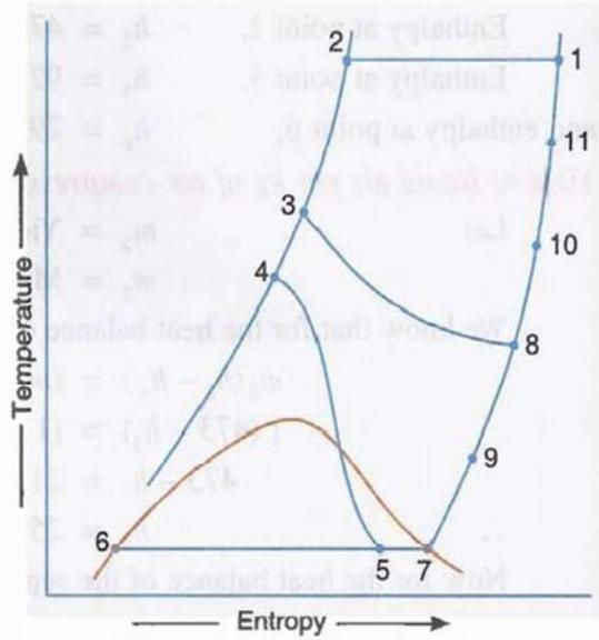
(b) T-s diagram for Claude air liquefaction system.
