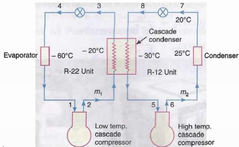
(a) Schematic diagram of a two-stage cascade refrigerating system.
