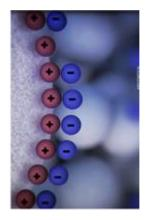
Ion exchange (IEX) chromatography is a technique that is commonly used in biomolecule purification. It involves the separation of molecules on the basis of their charge. This technique exploits the interaction between charged molecules in a sample and oppositely charged molecules in the stationery phase of the chromatography matrix.
