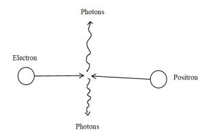
As the positron, after its formation, **slows down** as a result of **colliding** with **atoms** and doubles with the **electron**, which **leads to** the **annihilation** of the **positron** with the **electron**, and this process results in the <u>production of two</u> <u>photons with an energy</u> of **0.55 MeV** and this is called **annihilation rays**.
