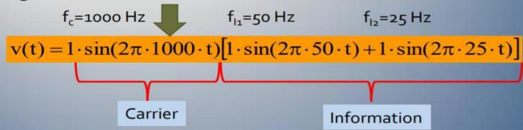
Modulation produces sums and differences of carrier and information frequencies
