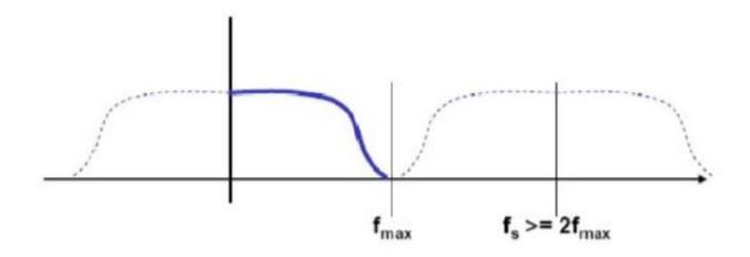
A signal that has energy to  $f_{max}$  must be sampled at a rate (2 x  $f_{max}$ ) or greater Sampling creates an "alias" copy of a signal
