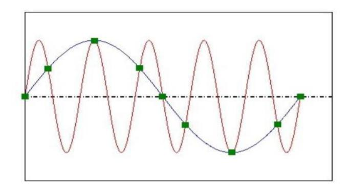
High frequency signal to be sampled by a low sampling rate may cause to "fold" the sampled data into a false lower frequency signal. This phenomena is known as *aliasing*.
