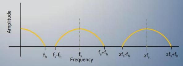
Sampling at less than 2fh causes aliasing and folding of sampled signals.
