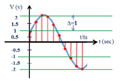
Signal amplitude of *range R* between  $X_{min}$  and  $X_{max}$  is divided into *L* quantization levels each of step size  $\Delta$
