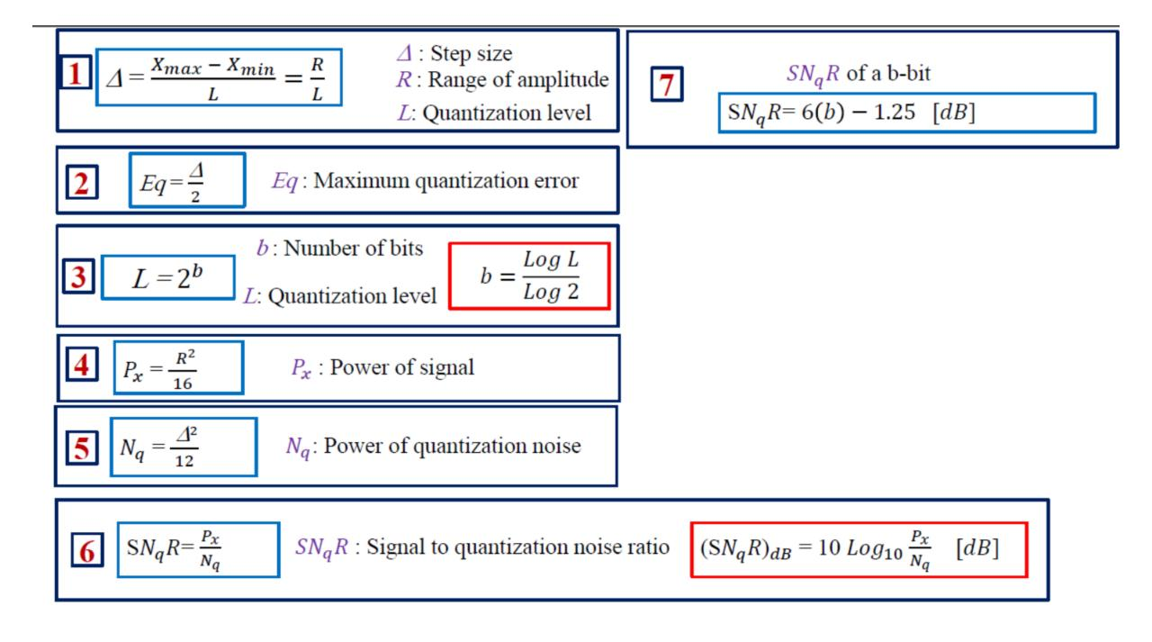
Ex:- An ADC is used to digitize the analog signal  $x(t) = \cos(1000 \pi t)$  at sampling frequency of  $f_s=2$  KHz. The ADC uses a 8- Levels quantizer and binary encoder the signal is  $P_x = 50$  mw.
