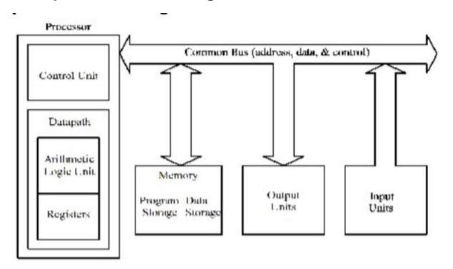
Although some computers used in data acquisition are highly specialized (the engine control computer in an automobile, for example), the computers normally used for data acquisition are quite standard and have the following components:
