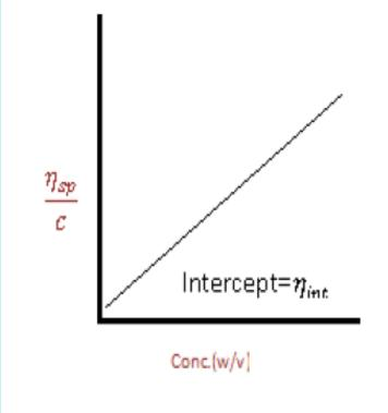
$\eta_{rel} = \frac{\eta}{\eta_0}$ we have to divide by  $\eta_w$  (viscosity of water)whatever the medium  $\eta_w$  viscosity of water is equal to **1 cp**.
