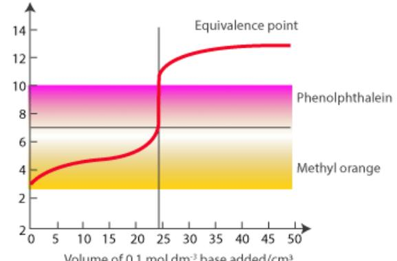
Titration of weak acid-strong base, adding  $0.1 \text{ mol dm}^{-3} \text{ NaOH(aq)}$  to  $25 \text{ cm}^3$  of  $0.1 \text{ mol dm}^{-3} \text{ CH}_3\text{CO}_2\text{(aq)}$
