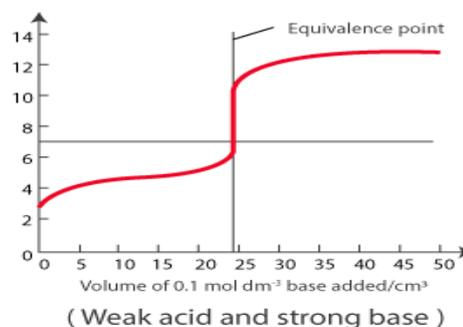
The pH does not change in a regular manner as the acid is added. Each curve has horizontal sections where a lot of bases can be added without changing the pH much. There is also a very steep portion of each curve except for weak acid and the weak base where a single drop of base changes the pH by several units. There is a large change of pH at the equivalence point even though this is not centred on pH 7. This is relevant to the choice of indicators for each type of titration.
