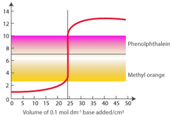
Titration of strong acid-strong base, adding  $0.1 \text{ mol dm}^{-3} \text{ NaOH(aq)}$  to  $25 \text{ cm}^3$  of  $0.1 \text{ mol dm}^{-3} \text{ HCl(aq)}$
