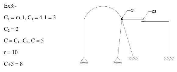
r > C+3, the frame is stable & indeterminate  $2^{nd}$  degree.
