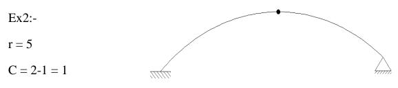
r > C+3, the frame is stable & indeterminate 1<sup>st</sup> degree.
