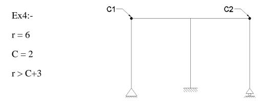
The frame is unstable because of internal geometric instability
