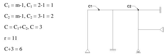
r > C+3, the frame is stable indeterminate 5<sup>th</sup> degree.
