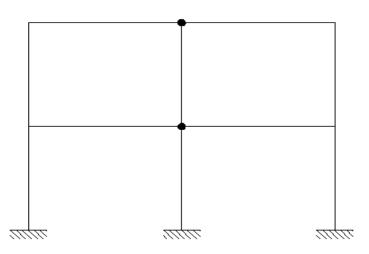
H.W2: Find the stability and determinacy of frame below
