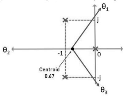
With angle  $\theta$ 2, one branch from s = 0 approaches to infinity and with  $\theta$ 1 and  $\theta$ 3, branches starting from -1+j and -1-j respectively, approach infinity.
