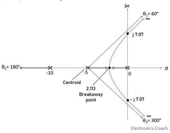
From the above sketch, the stability of the system can be analyzed that for **K** between 0 to 750 the system is completely stable as the complete root locus lies in the left half of s-plane. While at **K** = 750, the system is marginally stable.
