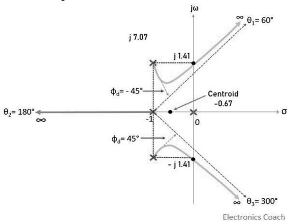
Now talking about stability, for **K between 0 to 4**, the roots are present on the left half of s-plane, representing a **completely stable system**.
