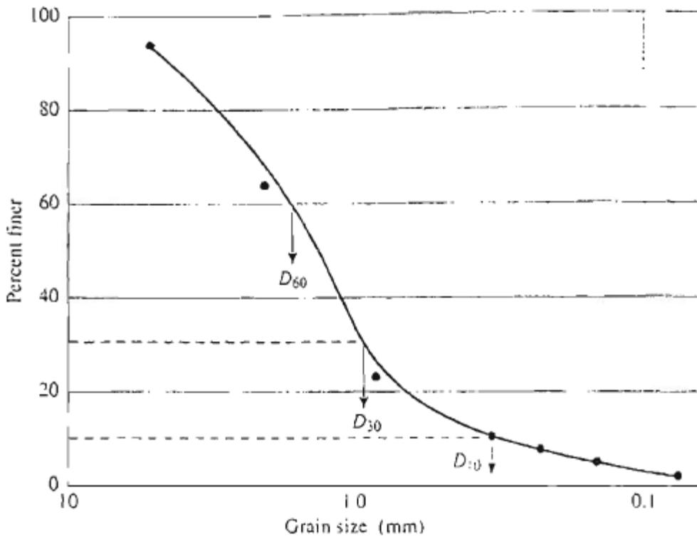
$$D_{60} = 1.41 \text{ mm} \quad D_{30} = 0.96 \text{ mm} \quad D_{10} = 0.41 \text{ mm}$$
