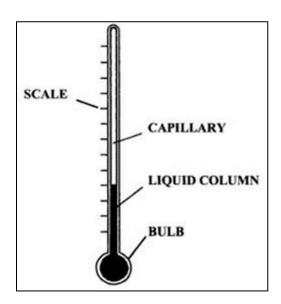
The smaller the diameter of the capillary, the greater is the sensitivity of the thermometer, a fever thermometer, which needs to show fractions of degrees, requires a capillary so small-less than 0.1 mm in diameter.
