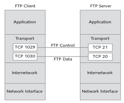
Figure 3-2 TCP port usage in FTP communications
