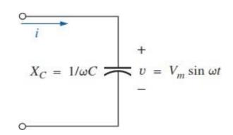
$$v = V_m \sin \omega t \Rightarrow \text{phasor form } \mathbf{V} = V \angle 0^\circ$$
