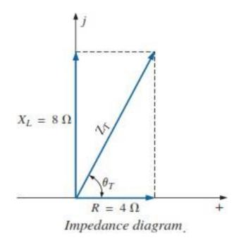
**EXAMPLE 15.8** Determine the input impedance to the series network in Fig. Draw the impedance diagram.
