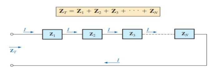
**EXAMPLE 15.7** Draw the impedance diagram for the circuit in Fig., and find the total impedance.
