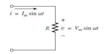
Since i and v are in-phase, the angle associated with i also must be 0°. To satisfy this condition,  $\theta_R$  must equal 0°.
