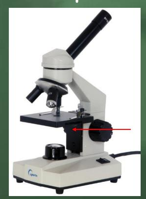
Coarse and fine adjustment knobs
