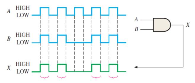
*A* and *B* are both HIGH during these four time intervals; therefore, *X* is HIGH.
