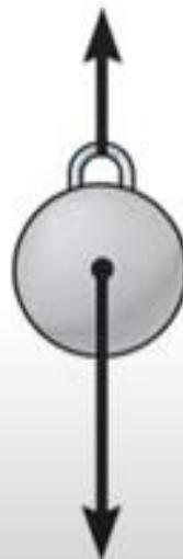
58.9 N (Weight or gravity acting on sphere)
