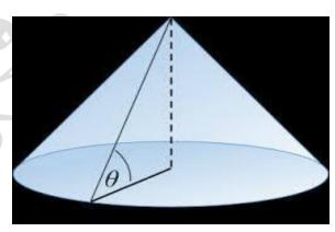
Powders with a low angle of repose flow freely, and powders with a high angle of repose flow poorly.
