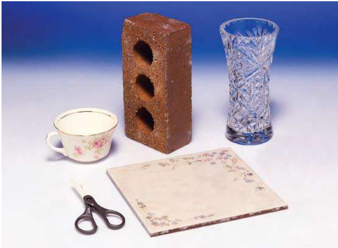
Figure 1. Common objects that are made of ceramic materials: scissors, a china tea cup, a building brick, a floor tile, and a glass vase.
