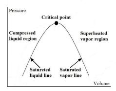
Property tables of other substances are used in the same manner. For each substance, the thermodynamic properties are listed in more than one table. In fact, a separate table is prepared for each region of interest such as the superheated vapor, compressed liquid, and saturated (mixture) regions.
