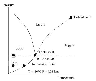
When the initial state of the system is -20°C and 0.613 kPa, the heating process results in increasing the temperature until it reaches 0.01°C. Further heating may result in some of the ice becoming vapor and some becoming liquid. Therefore at these conditions it is possible to have three phases in equilibrium. This point is called **triple point**; which is defined as the state in which the three phases of a pure substance may be present in equilibrium.
