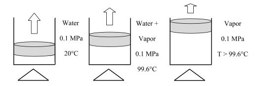
The term **saturation temperature** designates the temperature at which vaporization takes place at a given pressure. This pressure is called the **saturation pressure** for the given temperature. Thus, for water at 99.6°C the saturation pressure is 0.1 MPa, and for water at 0.1 MPa the saturation temperature is 99.6°C. For a pure substance there is a definite relation between saturation pressure and saturation temperature.
