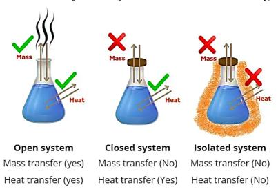
Open system (control volume): A thermodynamic system defined by a volume in space of interest. Both matter and energy can enter or exit an open system.
